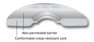
GLS flange models typically have a crowned flange mating surface. The gasket material characteristics determine the minimum sealing forces to create a seal. UPG gaskets combine a full density "skin" with a conformable core. This reduces the risk of media permeating the installed gasket, and provides the low stress-to-seal performance. The crowned surface can help build additional margin because of the stress concentration at the peak of the crown.
