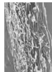
Non-woven material of GORE® Acoustic Vents as seen under magnification
