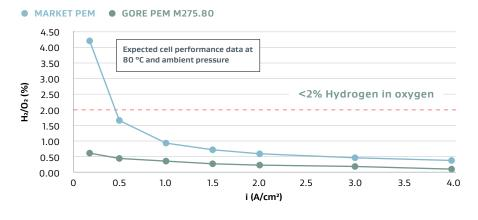
Gore's additive technology enables <2% hydrogen in oxygen concentrations over a wide operating range — even at low ampere/current densities.
