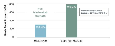
Gore's reinforced membrane offers >2x higher mechanical stability than non-reinforced membranes for extended system durability and reduced service intervals.
