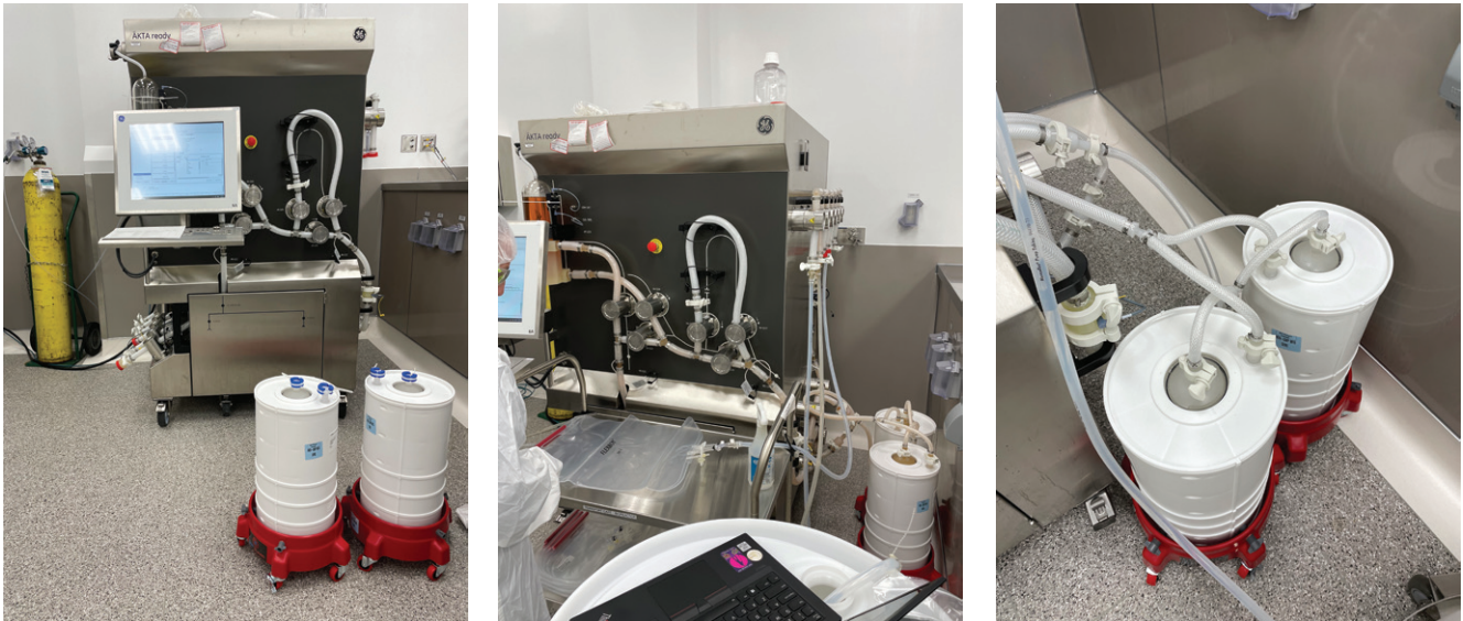
Fig. 2. Pictures of parallel manifolded 2 X 1 Liter Gore Devices with integration into chromatography system.
