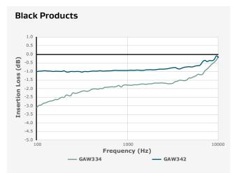
GAW342 has lower insertion loss than GAW334 and maintains a relatively flat response across the entire frequency range.
