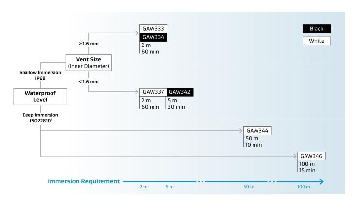
1) In compliance with ISO22810:2010(E) test method 4.3.2 Water resistance to overpressure.
