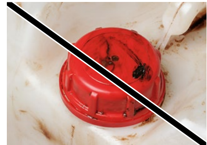
Venting holes blocked by liquid
