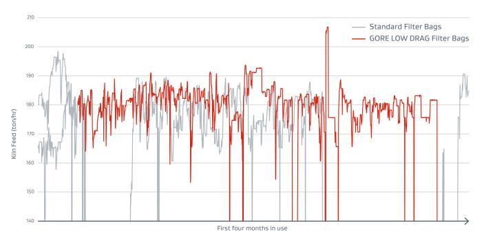
In the past, the plant reached peaks of 190 ton/hr for Kiln Feed. With GORE LOW DRAG Filter Bags they see an 8% increase (peaks of 206.1 ton/hr).
