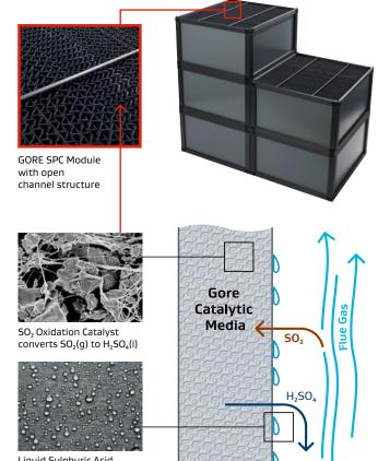
Liquid Sulphuric Acid expelled to media surface for gravity collection
