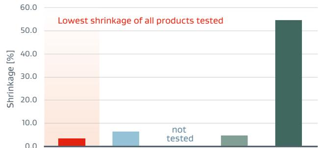
Gore's low shrinkage with excellent creep resistance can enable long packing life and enhance pump efficiency.
