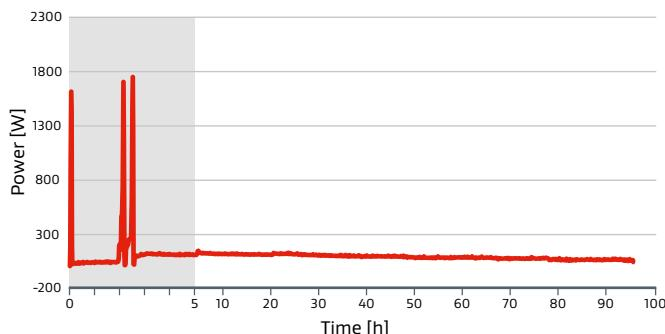
After initial break-in period, power consumption stabilizes at 85.2 W (after 5 adjustments)
