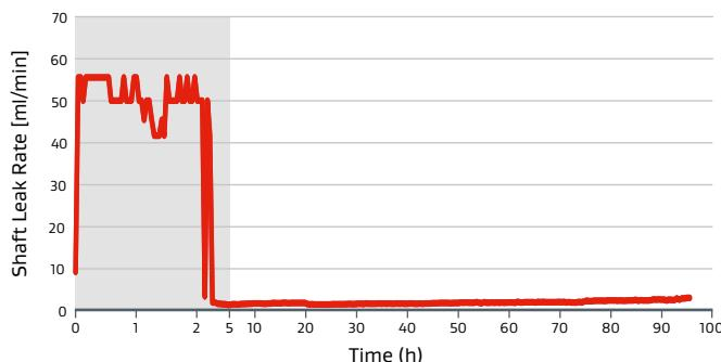
After initial break-in period, shaft leak rate stabilizes at 2.7 ml/min (after 5 adjustments)
