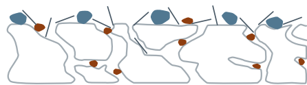
Tortuous path of non-woven material used in GORE® Acoustic Vents for Dust and Splash Applications
