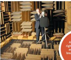
Above left and right: Steve Orfield and his recordbreaking anechoic chamber
