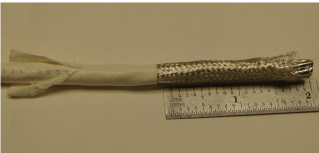
Figure 13: Exposing the braid
