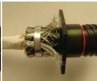
Figure 44: Attaching Band-It to receptacle
