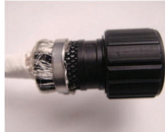
Figure 45: Trimming excess braid on plug
