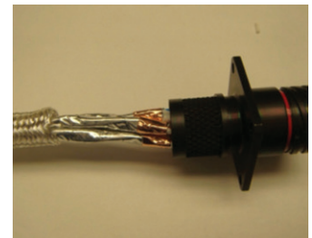
Figure 40: Inserting primaries into the connector
