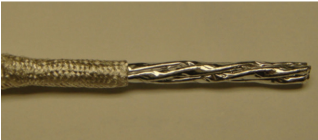
Figure 30: Exposing the foil
