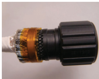
Figure 47: Taping the plug
