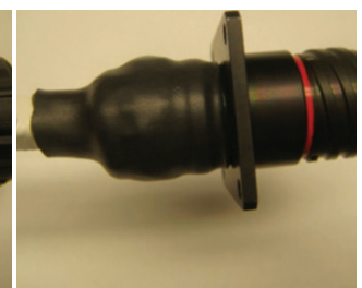
Figure 50: Shrinking tubing on receptacle
