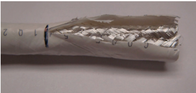
Figure 12: Slitting the cable jacket
