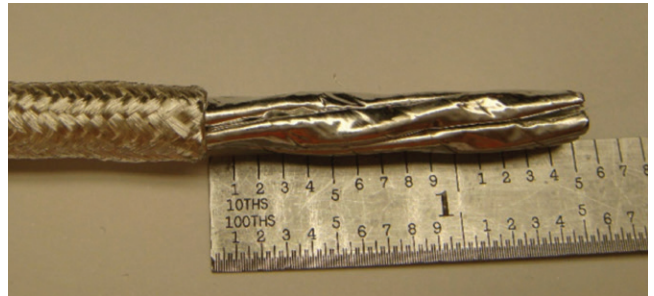
Figure 14: Exposing the foil
