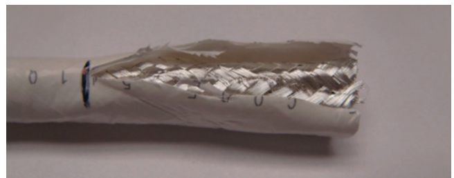
Figure 28: Slitting the cable jacket
