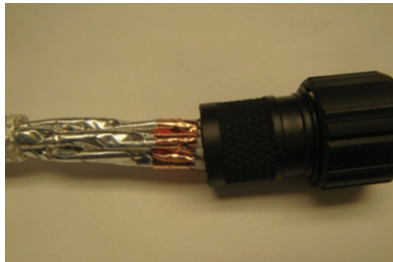
Figure 24: Inserting primaries into the connector
