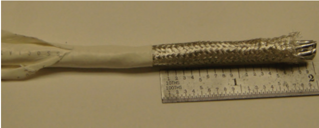
Figure 29: Exposing the braid
