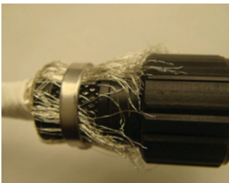
Figure 43: Attaching Band-It to plug
