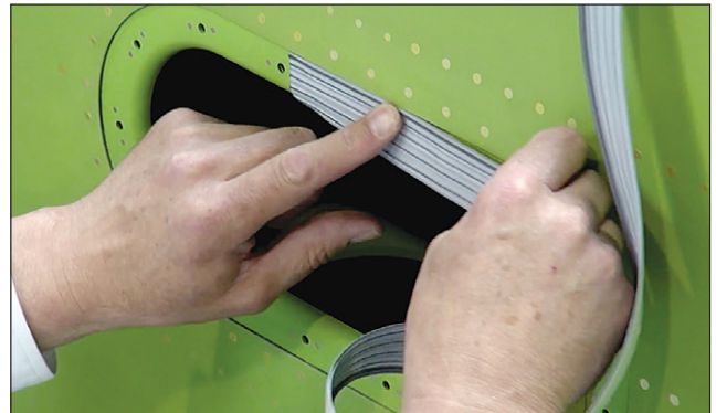
Figure 22: Positioning tape on frame
