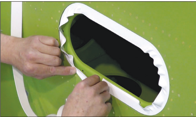
Figure 9: Forming a curve around frame
