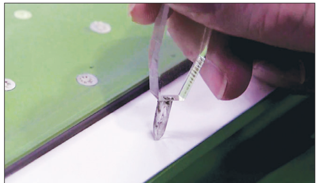
Figure 18: Forming a fastener opening
