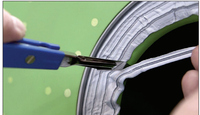
Figure 27: Trimming the tape around a curve
