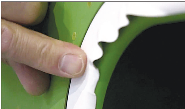
Figure 10: Wrapping the tape around curve
