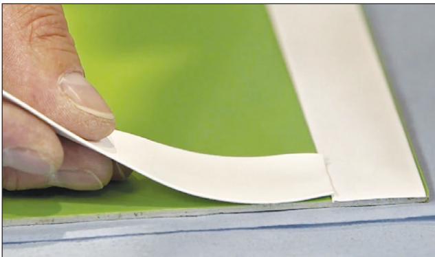
Figure 15: Sealing the two ends of the tape
