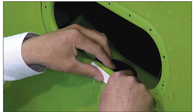
Figure 5: Positioning tape on frame
