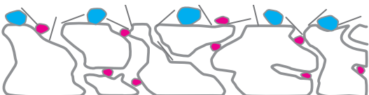
FIGURE 4: NON-WOVEN MATERIAL CAPTURES PARTICLES OF VARYING SIZE AND SHAPE BECAUSE OF ITS TORTUOUS PATH STRUCTURE.
