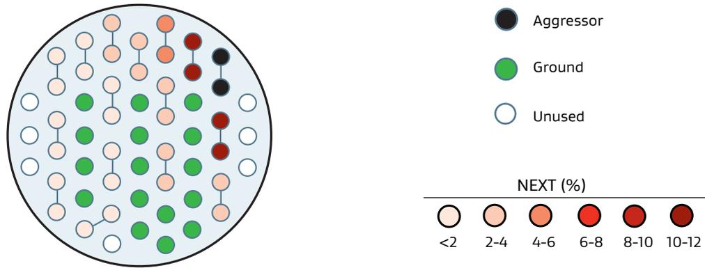
Figure 20 shows how pairs surrounding an aggressor pair can have edge-coupled crosstalk at about the same level as pairs that are directly adjacent.
