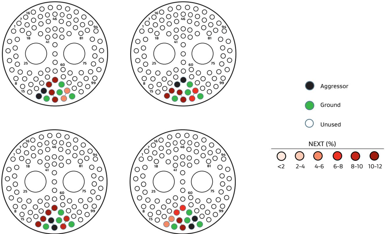
Figure 30: SAE AS6129, Size 25 Optimized Pinout Configuration
