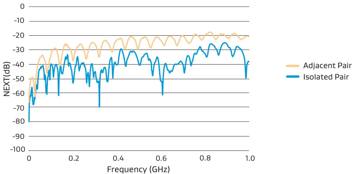
**Figure 17: Crosstalk Performance for 2 Sets of Pairs**
