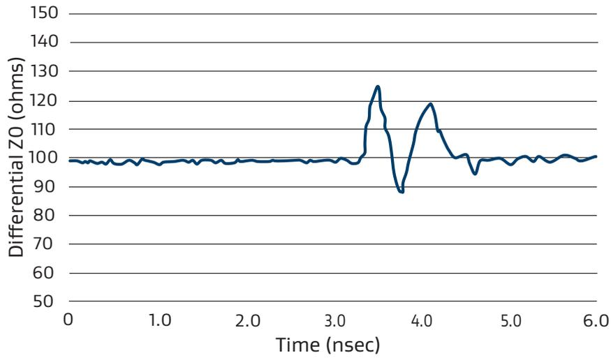
Because the relative positions of the signals and shields within each pair are essentially the same, results also indicated little difference in return loss performance between all four pairs (Figure 28). These values fail to meet the Cat6a wiring borderline for the ANSI/TIA 568-C industry standard, which means that the connection will likely be out of specification when using this pinout and could be worse depending on termination techniques
