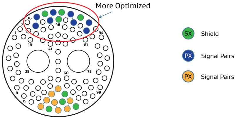
Figure 31: Crosstalk Performance for SAE AS6129, Size 25 Optimized Pinout Configuration
