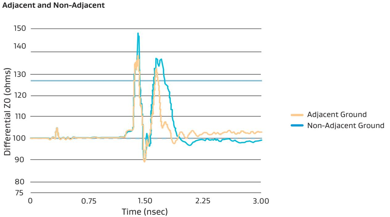
Figure 12: Return Loss for Adjacent and Non-Adjacent Shield Connections
