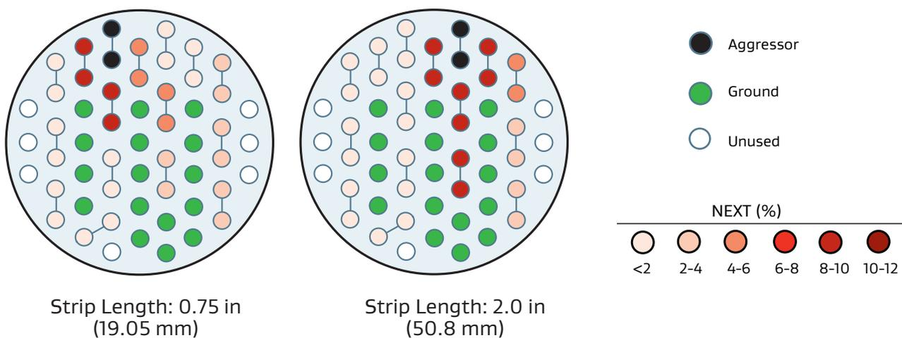
Crosstalk mappings of the remaining victims in the MIL-DTL-38999 open pin field connector system are shown in Figure 23. Based on these results, Gore concluded the following:
