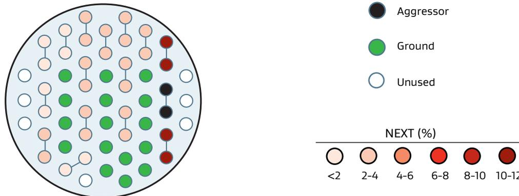
Figure 21 shows how adding separation and including ground pins between pairs can reduce crosstalk; however, it does not maintain it below 6 percent. Adding ground pins can take up significant connector real estate and with additional termination time for a cable assembly.
