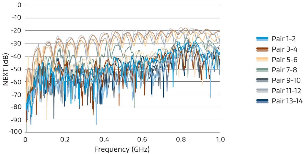
If crosstalk limit lines are added based on Cat6a requirements for 10-Gb/s Ethernet data transmission, results clearly show that some interactions exceed the allowable crosstalk levels for reliable data transmission (Figure 15).
