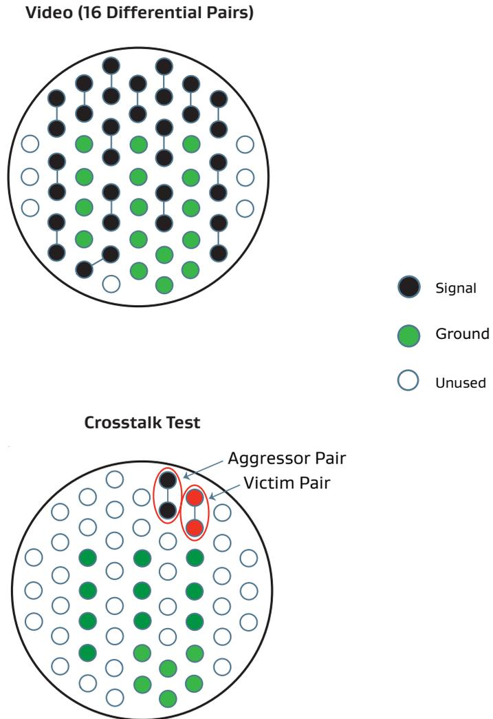
Gore applied an aggressor signal to each signal pair in the connector system and measured crosstalk for 15 victim pairs. The results yielded 15 crosstalk measurements in the frequency domain for each aggressor pair (Figure 14).
