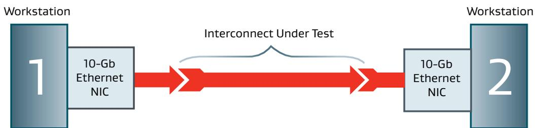
The data is monitored at each end of the link tracking retries, packet drops, and packet errors to see how various transmission lines affect the performance of the link. The system also detects when the cable assembly degrades the signals enough to cause autonegotiation to 1 Gb/s or even 100 Mb/s, which allows for comparisons in network performance between different physical interconnects.
