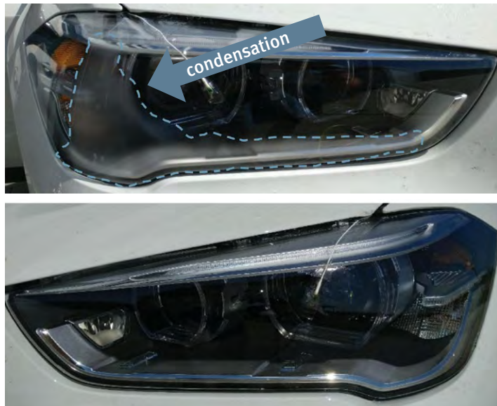
Figure 10: Top – Reference headlamp (no CMD) with condensation; Bottom – Headlamp with CMD with no condensation after spray event.
