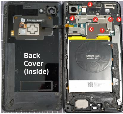
**Figure 9:** Google Pixel 3XL with back cover removed. Existing air gap thickness measured by conformable polymer at seven locations shown.
