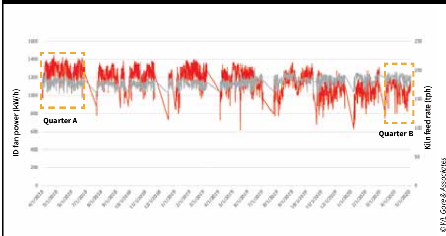
Figure 1: two significant three-month periods (Quarter A and Quarter B, respectively) in the cement plant's production after installation of the Gore filter bags
