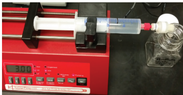
Figure 2. Semi-automated purification using a syringe pump and a 30 mL syringe attached to a 1.0 mL GORE Protein Capture Device
