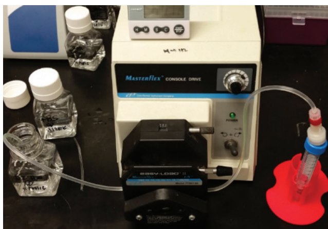
Figure 3. Semi-automated purification method using a peristaltic pump, attached to a 1.0 mL GORE Protein Capture Device
