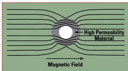
▲ Fig. 2 Magnetic field shielding.
