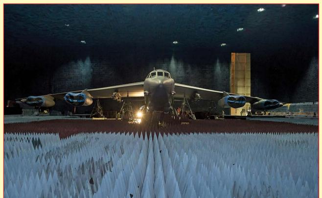
▲ Fig. 2s Interior of the anechoic chamber with a B-52 Stratofortress staged for testing. Pyramidal objects in foreground are electromagnetic absorbers. Source: Edwards Air Force Base
