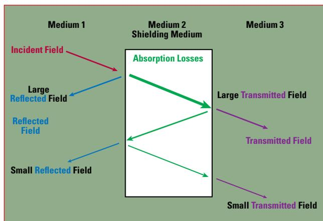
▲ Fig. 1 Schellkunoff model of E-field shielding. Source: York EMC Services.
