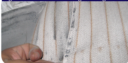
Figure 6: examination of bag stitching
