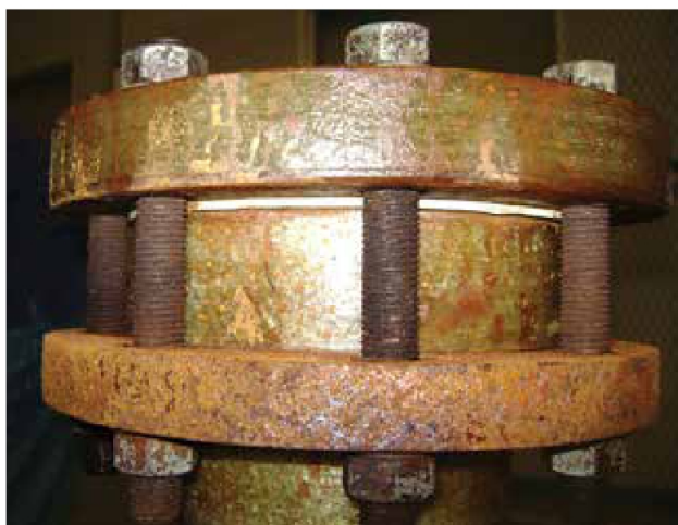
After chemical test - Flange reveals no chemical attack after 1000 hours of 37 per cent HCl exposure
