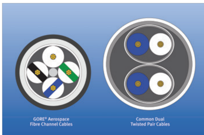
FIGURE 28: LOW-DIELECTRIC CABLE GEOMETRY
