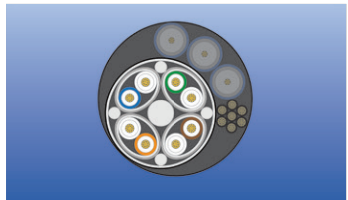
FIGURE 36: GORE'S SINGLE-LINK CABLE IN STANDARD DVI HARNESS CROSS-SECTION
