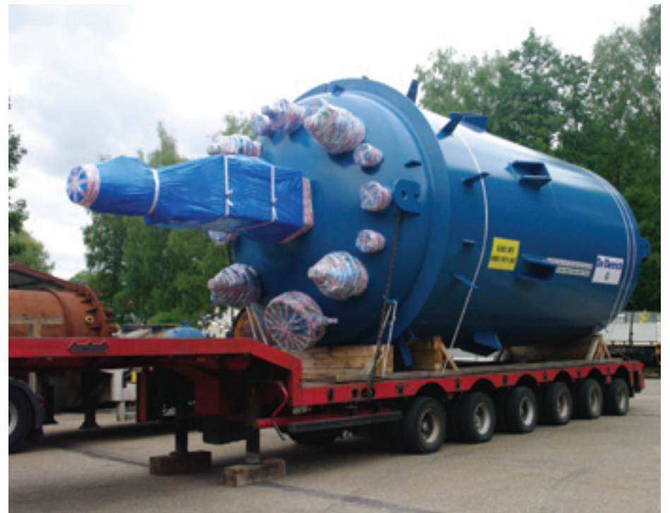
Fig. 2: Example of a large scale glass-lined steel vessel.
