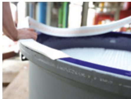
Fig. 1: Close-up of glass-lined steel flange.
