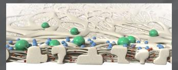
Non-woven material captures particles of varying size and shape because of its tortuous path structure.
