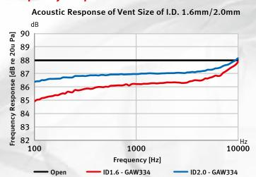
The test represents the response from a typical MEMS microphone system in Gore laboratory with representative sample size. Performance may vary depending on the design of the device.
