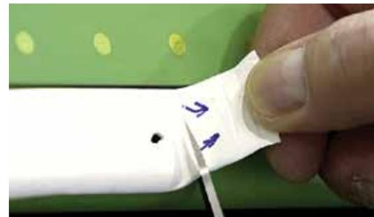
Figure 11: Removing the damaged section
