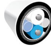
Part Number: 104 High Frequency Signal Cable CAN BUS impedance: 100 Ohm +/- 10 Ohm 2x AWG 24 shielded white, blue Ratings: 300V rms Dimensions: 4.9 mm +/- 0.1 mm (0.193 in +/- 0.004 in)
