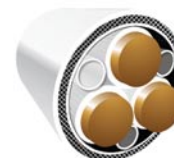
Part Number: 112 Shielded Power Cable 3x AWG 14 shielded white, black printed 1-3 Ratings: 600V rms Dimensions: 7.1 mm +/- 0.1 mm (0.280 in +/- 0.004 in)
