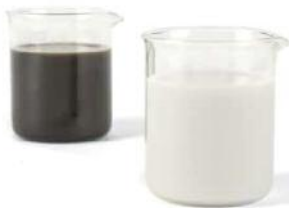
Figure 5. Used compressor washing fluids from two adjacent GE LM6000 turbines. Left: 1st turbine after 1450 operating hours with F9 rated nano fibre filters. Right: 2nd turbine after 2500 operating hours with the membrane based Gore filter
