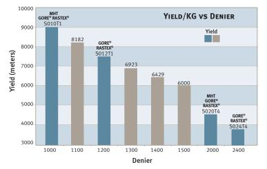
Because of its high yield, lower denier MHT GORE® RASTEX® Sewing Thread can provide lower cost per meter than many higher denier threads.
