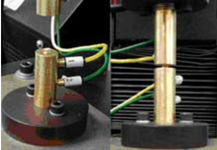
Gore's micro-ohmmeter with four-point probe measures the amount of resistance that passes through all layers of the ground pad.
