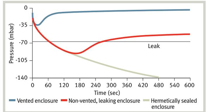
In non-vented housings, 70 mbar (1 psi) of pressure causes seals to leak after repeated temperature cycles. Vented housings equalize pressure and prevent seals from leaking.
