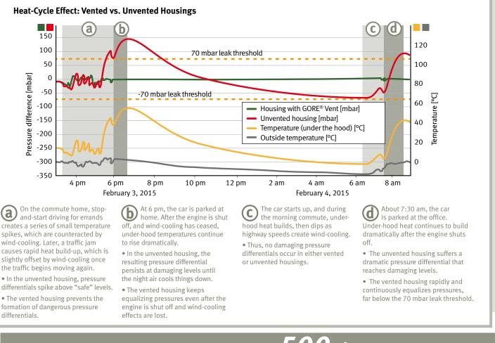
Just 2 engine start-ups/shut-offs per workday will create more than **500 dangerous** under-hood **temperature spikes** per year. In unvented housings, the resulting pressure differentials can create premature seal failure. With GORE® Automotive Vents, these pressure differentials are rapidly and continuously equalized before they can stress seals and threaten the electronics within.
