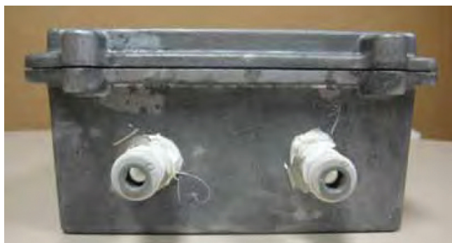
Figure 2: Aluminum housing with ports installed for pressure and temperature probes
