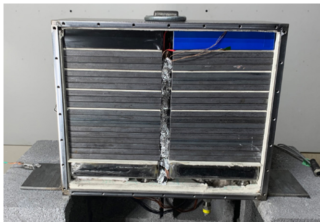
Figure 2: The fully loaded enclosure with the cover removed
