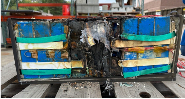
Figure 8: ONE Battery Module After Thermal Runaway Propagation Test, Showing the Prevention of Thermal Runaway to Adjacent Cells Enabled by GORE Battery Insulation Technology
