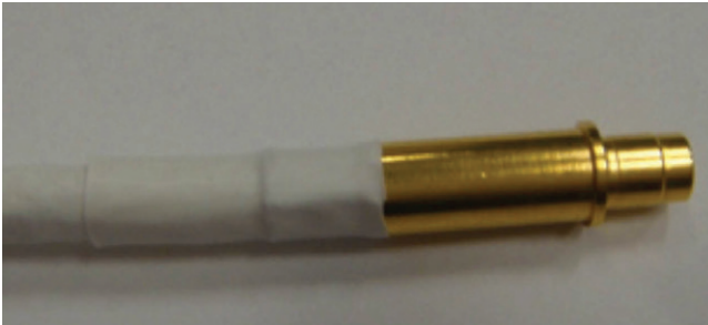
Figure 63: Shrinking tubing on crimp pin
