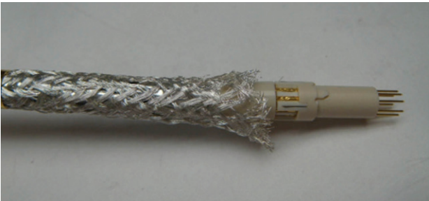
Figure 27: Returning the braid
