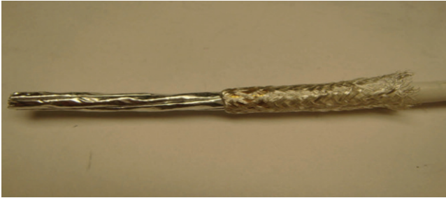
Figure 40: Exposing the foil
