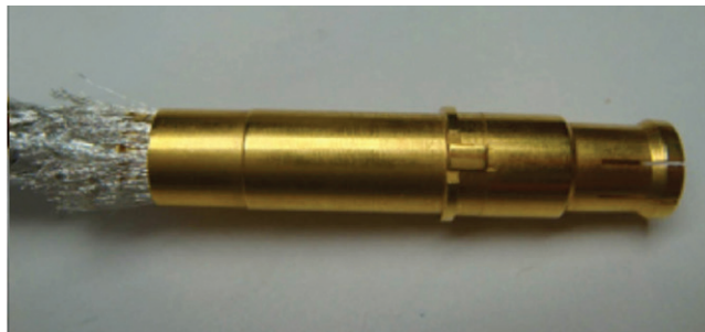
Figure 31: Installing outer body
