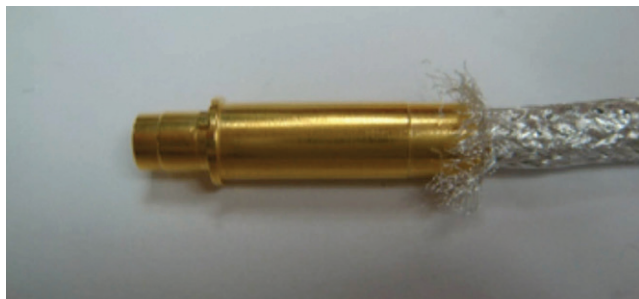
Figure 55: Installing outer body
