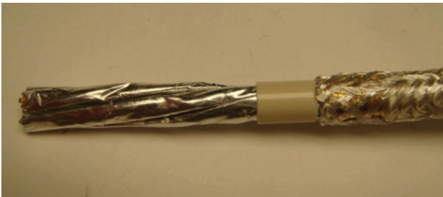
Figure 41: Sliding plastic bushing onto cable
