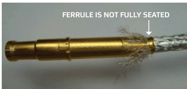
Figure 56: Ferrule not fully seated
