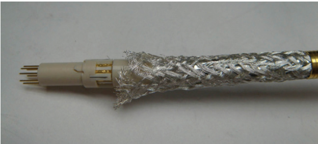
Figure 51: Returning the braid
