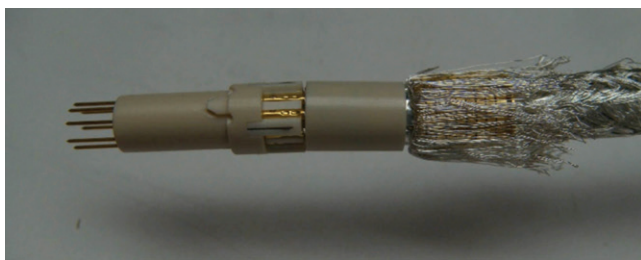
Figure 53: Brushing the braid
