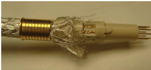
Figure 28: Returning the ferrule
