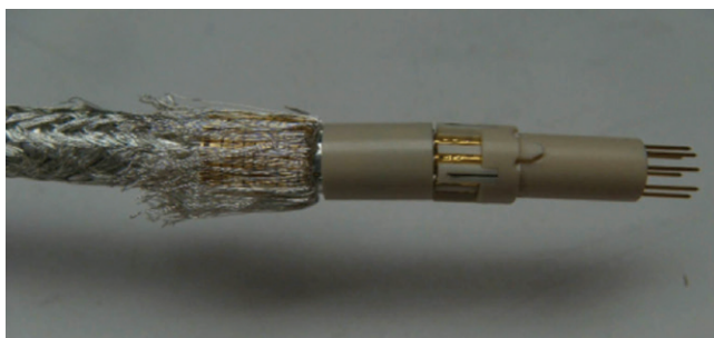
Figure 29: Brushing the braid
