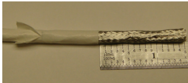
Figure 13: Exposing the braid
