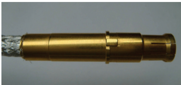
Figure 33: Trimming the braid
