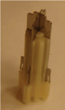
Figure 22: Inner insulator with metal spacers
