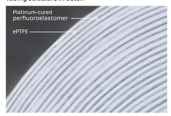
Unlike conventional tubing, Series PFL is manufactured with a patented composite structure of platinum-cured perfluoroelastomer and expanded polytetrafluoroethylene (ePTFE) for increased reliability with aggressive chemicals in peristaltic pumps.
