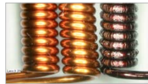
Polyamide enameled wires become brittle and crack.
