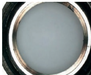
Fig. 9/10: Visual inspection of a GORE® Protective Vent after 8 years
