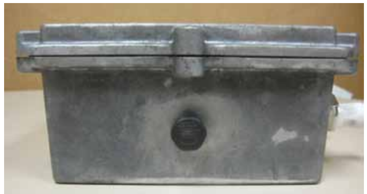
FIGURE 3: ALUMINUM HOUSING WITH GORE® PROTECTIVE VENT INSTALLED
