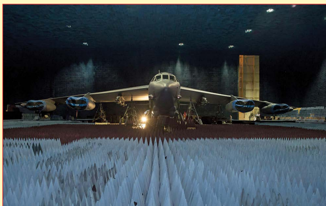
▲ Fig. 2s Interior of the anechoic chamber with a B-52 Stratofortress staged for testing. Pyramidal objects in foreground are electromagnetic absorbers. Source: Edwards Air Force Base
