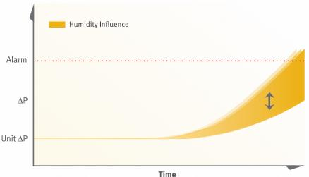
Trend monitoring of filter  $\Delta P$  is the most reliable way to decide when to replace filters. The chart on the left depicts the typical  $\Delta P$  profile over the service life of a GORE® Turbine Filter. When the ΔP trends upward and the influence of humidity grows, it is time to plan for filter replacement.
