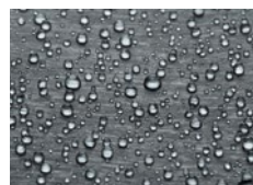
Liquid Sulphuric Acid expelled to media surface for gravity collection
