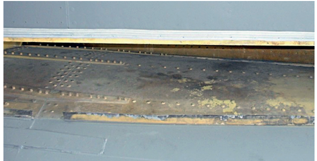
Figure 4: Fin-to-Body Fairing Panels
