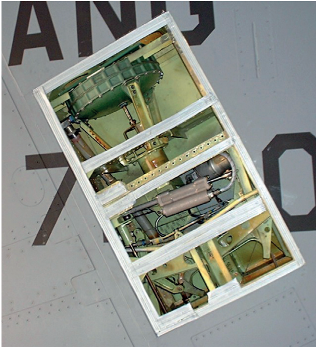
Figure 2: Q Spring and Control Quadrant Access Panels
