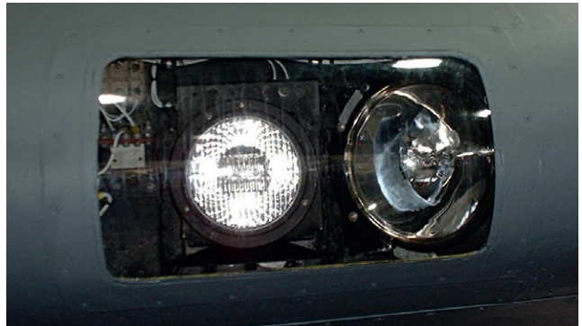
Figure 5: Landing Light Cover
