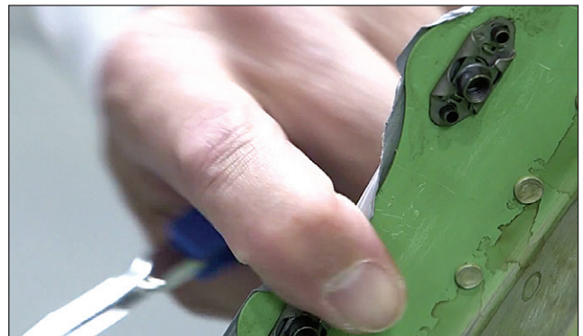
Figure 23: Wrapping tape along edges
