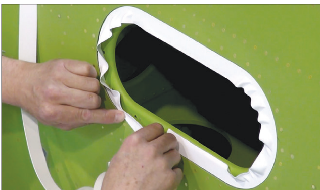
Figure 9: Forming a curve around frame
