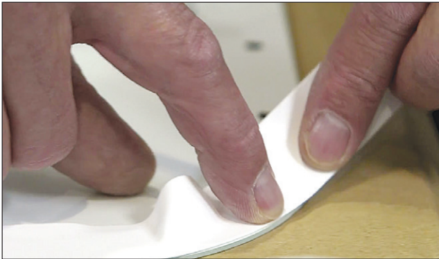
Figure 8: Forming a curve around panel
