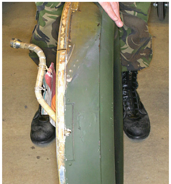
Figure 4: Chafing damage to engine inlet D-ring cowl at mating surface.
