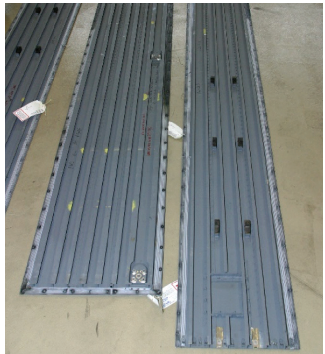
Figure 7: GORE® SKYFLEX® Aerospace Tapes, 110 Series installed on floor panels.
