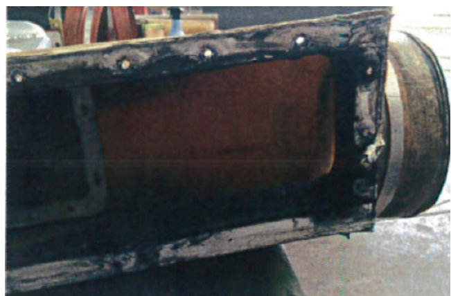
Figure 2: Repair required for missing or damaged sections of Gore's 200 Series (part number GUA1302-1).
