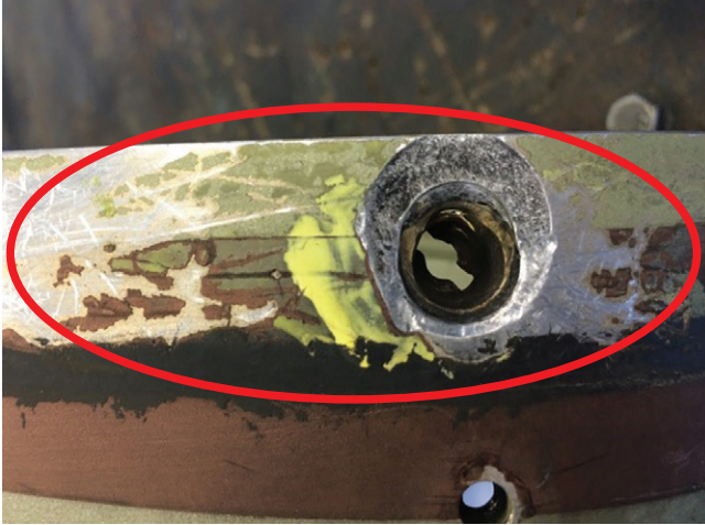
Figure 1: Typical example of chafing damage on tail boom structure around the fastener receptacle.
