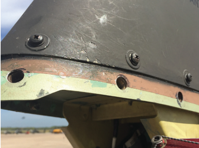
Figure 5: GORE® SKYFLEX® Aerospace Tapes, 730 Series removed from test aircraft.
