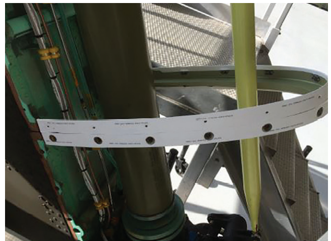
Figure 4: GORE® SKYFLEX® Aerospace Tapes, 730 Series installed on lower rib assembly.
