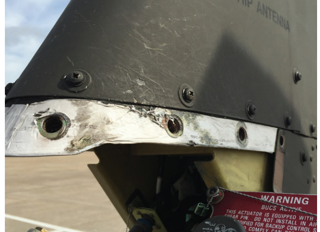
Figure 6: GORE® SKYFLEX® Aerospace Tapes, 730 Series installed on test aircraft reveals frictional stress absorbed by material.
