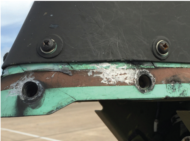
Figure 7: No tape installed on control aircraft, reflecting wear on unprotected surface.
