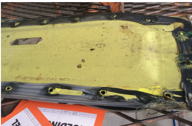
Figure 2: Material torn away from fastener holes and corners, excessively compressed (black), and separating from panel
