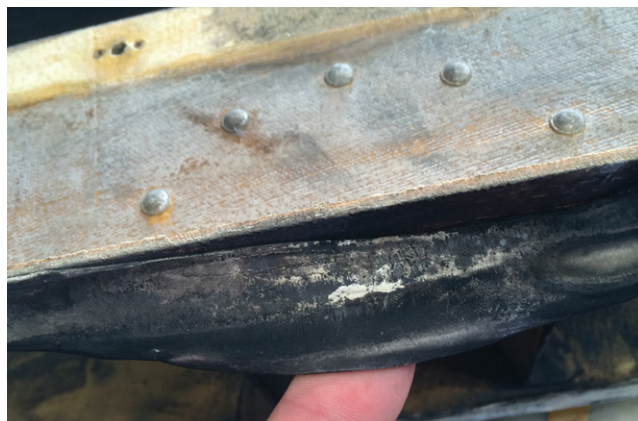
Figure 6: Material blackened and stiffened
