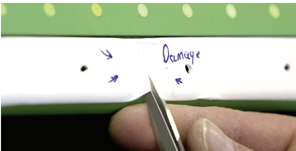
Figure 9: Slitting the damaged section
