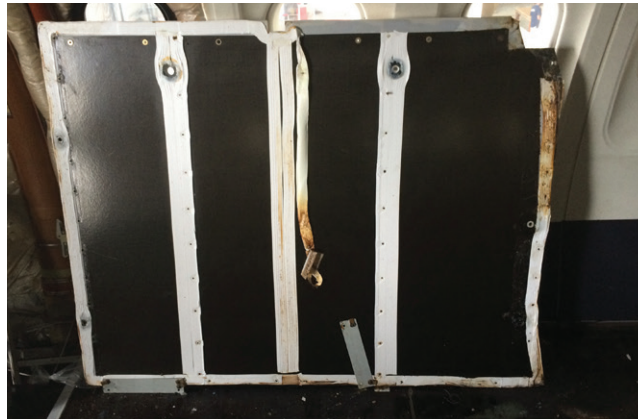
Figure 4: Material torn away from fastener holes and corners, separating from panel, and gaps in sealant
