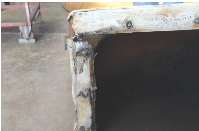
Figure 3: Material excessively compressed and worn
